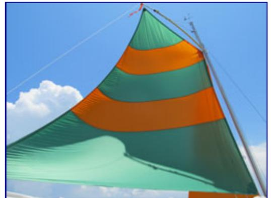
I fabricated a lightweight gaff by modifying a fiberglass/aluminum telescoping pole found in Home Depot. The gaff is bent slightly because some weight of the boom (and stowed main) is supported by the adjustable self-standing leech line (shown in photo), which also serves as a topping lift to help the boom clear the gallows when tacking.
