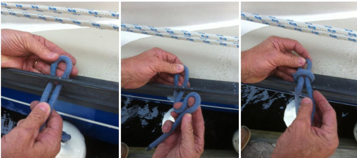
To release, I simply pull on the loose end of the line and the fender is hanging in my hand. Obviously, if the line diameter is small enough in relationship to the hole, it would slip through. I have also used this method to make quick-release docklines when the occasion called for it. As always, thanks for your great magazine.
