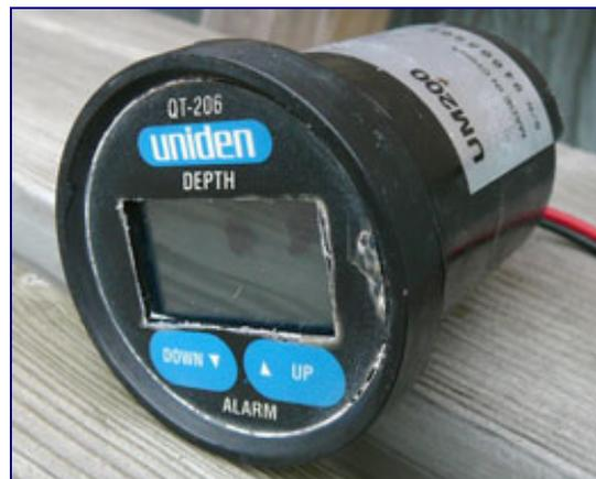
You should be good for several more years of clear viewing! It is important to keep moisture out of the depth sounder or you will start to have blacked-out pixels in the LCD display.
