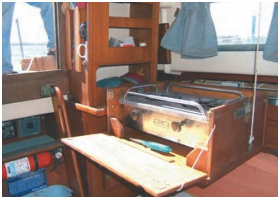
**Without putting too fine a point on it, galleys were not the strong suit of the Tritons. Jack added a stove and vital cooking space by installing a Luke stove which folds up and out of the way when not in use, above and far left. The drop-down table, center left, and counter space, below left. Notice the fine woodworking throughout. Jack is a capable finish carpenter.**
