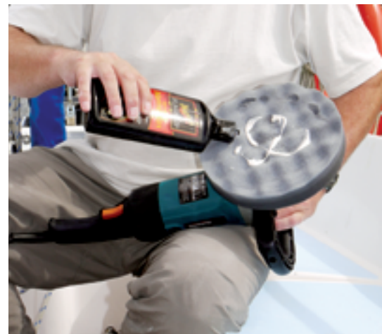
A wool pad, at left, is best for applying and working with rubbing compounds and polishes, and using a variable-speed rotary polishing machine almost goes without saying. After the compounding and polishing stage, wiping the surface with a cloth dampened with detailing spray, above center, removes residue. Wax should be applied sparingly, and a waffle-finish foam pad works well for applying it, above right. Peter's toil begins to show results, below.
