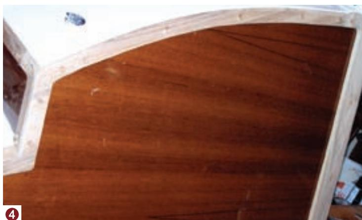
the inside. We used ¼-inch plywood cutouts to fill the ports and applied tacky-tape along with the poly to accomplish the seal.
