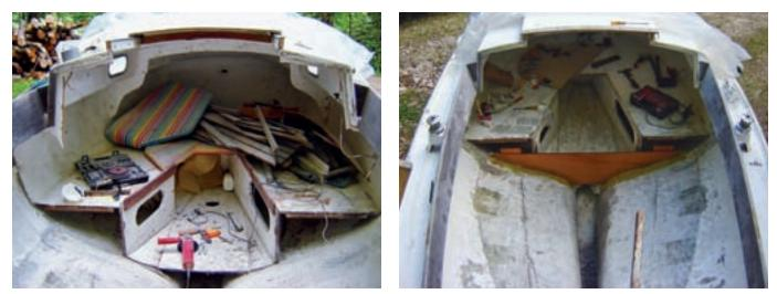
By the time Kegan had removed all the decayed wooden parts, the boat was looking rather bare, at left. At last reconstruction began, with the base for the main bulkhead, at right.
