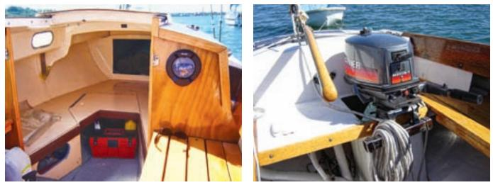
Kegan spent an entire summer working on the boat and launched her the following spring, by which time she was gleaming, at left. The venerable Mariner outboard, at right, was a gift — Kegan just had to get it working. All it needed was gas and a water-pump impeller.
