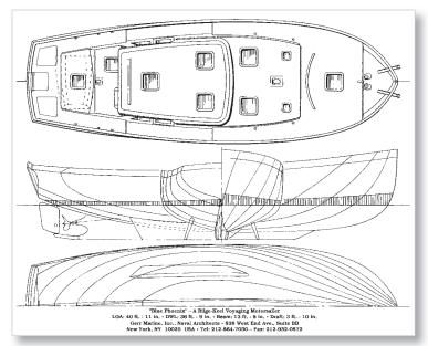
With the interior sketched out, it's time to define the shapes of the hull and the deck structures, at left, while keeping in mind the desired appearance of the finished design, below. That takes more pleasant hours of noodling.
