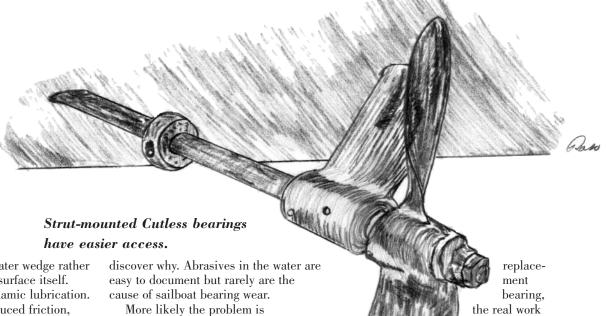
up and is riding on a water wedge rather than the nitrile rubber surface itself. This is called hydrodynamic lubrication. It makes for greatly reduced friction, reduced heat, and long bearing life.
