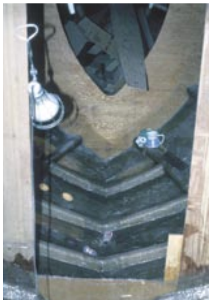
To stabilize the keel, Dave built box-section keel floors using \frac{3}{8} -inch marine plywood, sheathed in fiberglass, then laminated to the hull, above. A hard dodger and fiberglass doghouse, below left, prevented seas from entering the cabin. Launch day, below right.
