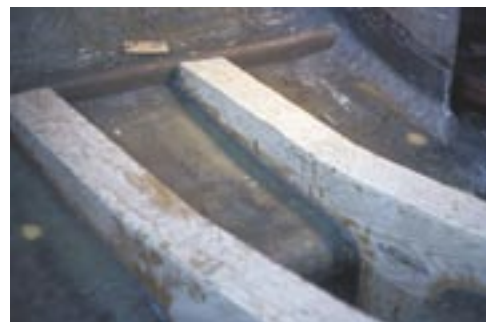
To stabilize the keel, Dave built box-section keel floors using \frac{3}{8} -inch marine plywood, sheathed in fiberglass, then laminated to the hull, above. A hard dodger and fiberglass doghouse, below left, prevented seas from entering the cabin. Launch day, below right.
