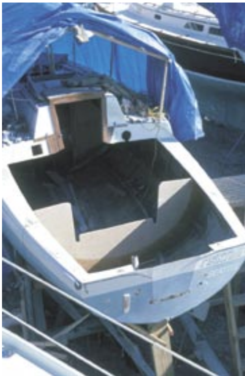
The new, aft, thwartship bulkhead, above. The cockpit getting primed for paint, at right. Note the wide gunwales and the stern deck with its hatch (not installed). Installing deck hardware, below.
