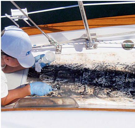
A tedious part of the project was filling the old screw holes with epoxy, above. Heidi and Terry did this before power sanding the deck in preparation for the application of a layer of fiberglass cloth in epoxy resin, near right. After the epoxy had cured in the sun for a week, they sanded it fair, far right, before applying the non-skid finish.
