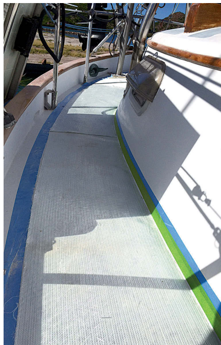
A tedious part of the project was filling the old screw holes with epoxy, above. Heidi and Terry did this before power sanding the deck in preparation for the application of a layer of fiberglass cloth in epoxy resin, near right. After the epoxy had cured in the sun for a week, they sanded it fair, far right, before applying the non-skid finish.
